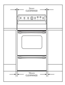
3. Anti tip brackets are supplied with the accessories, so that the product can be secured to the wall to prevent it from tipping over.
